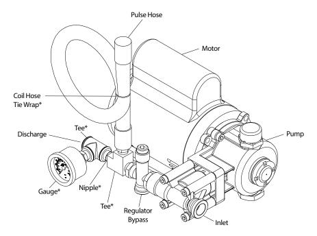
\*Not Supplied With Motorized Pump Unit
