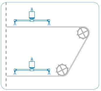
Spray arm assemblies can be mounted above the production side of belt, on the bottom side of belt, or both depending on belt type and cleaning required. Catch basin can be installed to capture product from the belt.
