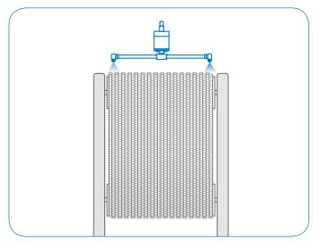
A single spray arm can be used to clean belts that are 4-24" in width.
