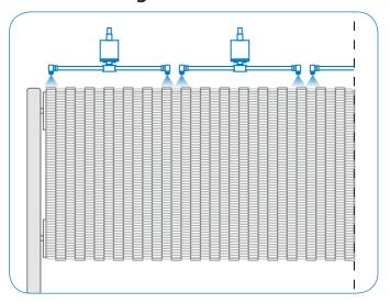
Two or more rotor spray arms can be configured to cover belt widths greater than 24".
