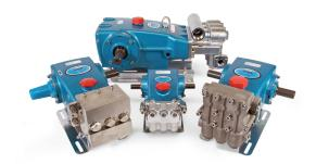
Cat Pumps liquid  $CO_2$  series of pumps feature modifications to accommodate the unique properties of liquid  $CO_2$ . Specialty seals handle low lubricity and low temperature that liquid  $CO_2$  applications require. Pump manifolds are modified to allow higher inlet and discharge pressures up to 7,000 psi (483 bar). Drive-end and manifold material combinations are available to cover a wide flow range from 0.34 to 50 gpm (189 to 27,800 lbs/hr).
