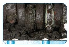
· Contaminated drive-end shown, due to loss of oil lubricity leading to component discoloration and failure
