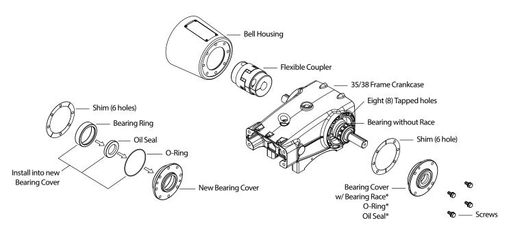
\*Remove three (3) items and install into new Bearing Cover
