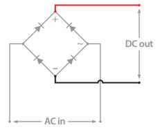
Red wire from 8136 motor connects to (+) terminal. Black wire from 8136 motor connects to opposite corner.
