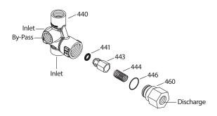
To convert 7537, 7542 unloaders to relief valves 7537.100, 7542.100. Remove items 441, 443 and 444. Reinstall items 446 and 460.
