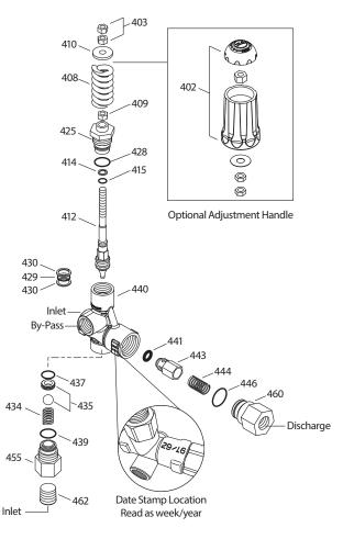
To convert to optional handle assembly, remove items 403 (quantity 2), 410 and 409. Then reassemble as shown in insert.
