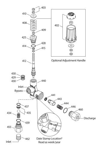
To convert to optional handle assembly, remove items 403 (quantity 2), 410 and 409. Then reassemble as shown in insert.
