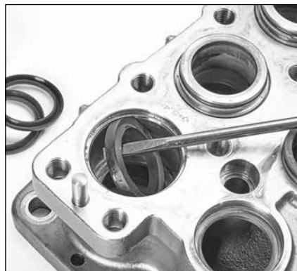
1.21 Use a large flat tip screwdriver to remove female adapter from each seal chamber.
