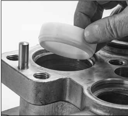
1.28 Install male adapter into each seal chamber with "V" shape facing down.
