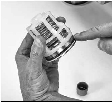
2.10 Lubricate O-ring and backup ring on valve seat.
