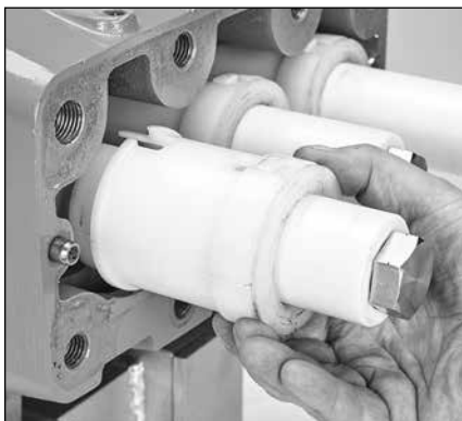
1.33 Remove seal retainers with wicks.
