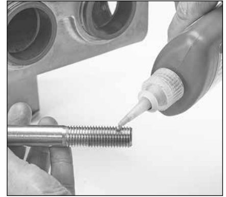
1.49 Apply Loctite®242® to four (4) M16 x 50 and two (2) M16 x 120 HSH screws; insert screws into inlet manifold and hand tighten. Remove two (2) studs.
