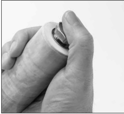
1.42 Insert plunger retainer assemblies into ceramic plungers.
