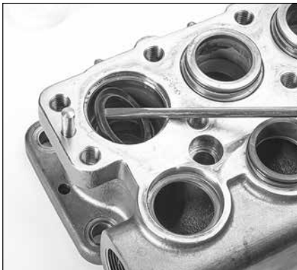
1.20 Use a large flat tip screwdriver to remove the pair of black V-packings from each seal chamber.
