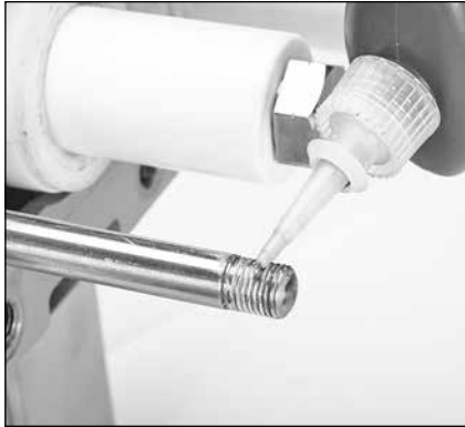
1.45 Place a drop of Loctite®242® on the end of each plunger rod.
