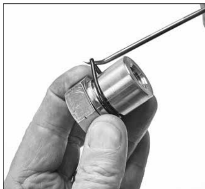
1.40 Use a pick to remove backup ring, O-ring and gasket from plunger retainer.
