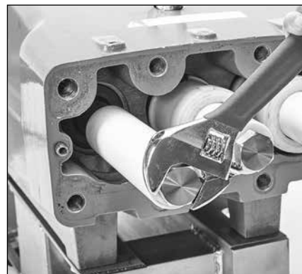
1.35 Use an adjustable wrench or 30 mm combination wrench to loosen the plunger retainers.
