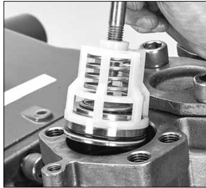
2.11 Hand thread in M12 HSH screw into top of valve retainer. Place new preassembled valve assembly into each valve chamber.
