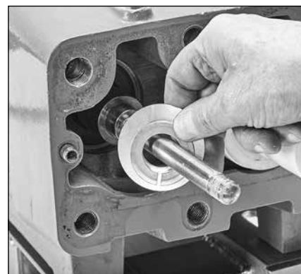
1.38 Remove keyhole washer and barrier slinger.
