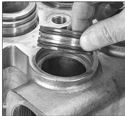
1.32 Install inlet spacer into each inlet chamber.
