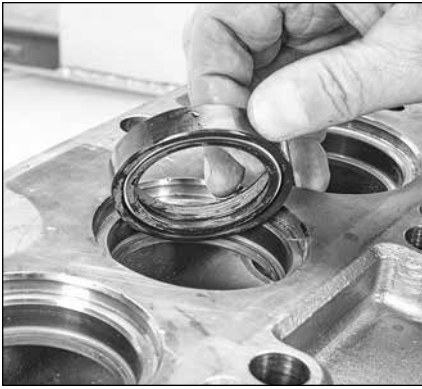
1.24 With crankcase side of inlet manifold facing upwards, install groove side facing down and press into place.
