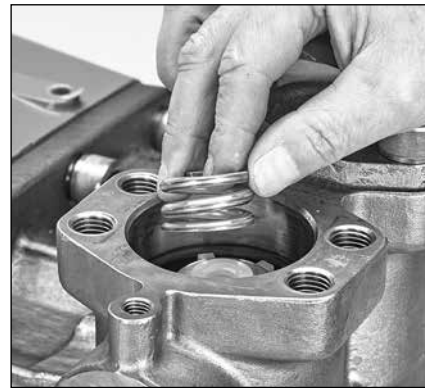
2.14 Install coil spring onto spring washer.
