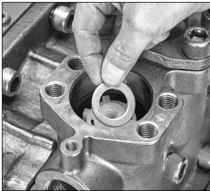
2.13 Install spring washer onto spring retainer.
