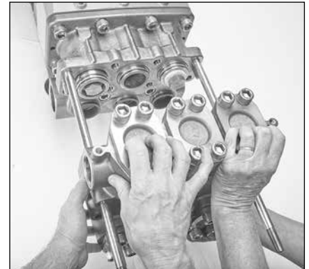
1.52 With a helper, line up the holes on discharge manifold with studs and slide over ceramic plungers and press discharge manifold against inlet manifold.
