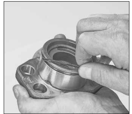
2.15 Install and lubricate new O-ring onto each valve plug.
