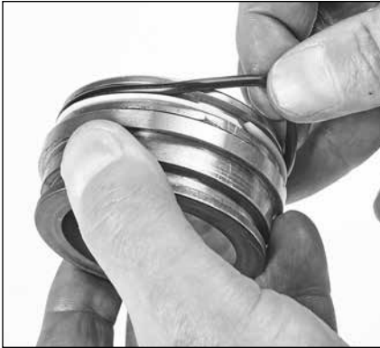
1.29 Install backup ring and then O-ring on both ends of V-packing spacer.
