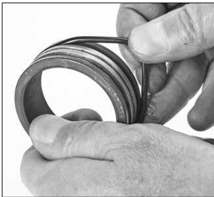
1.31 Install O-rings on both ends of inlet spacer.
