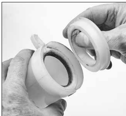
1.34 Separate the 2-piece retainer and remove the wick. Inspect all three (3) parts for damage and replace as needed.
