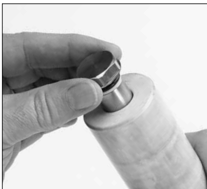
1.39 Remove plunger retainer from ceramic plunger.
