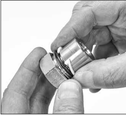
1.41 Install gasket, O-ring and then backup ring onto each plunger retainer.
