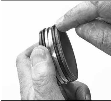
1.17 Inspect O-rings for damage.
