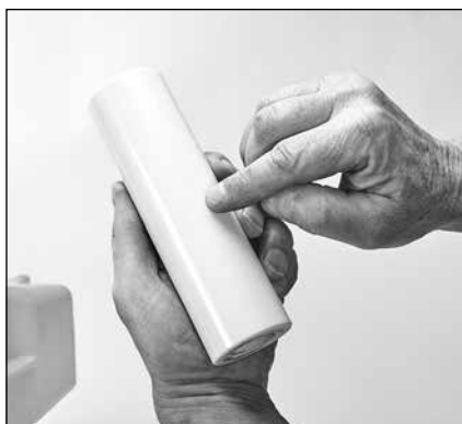
1.37 Inspect ceramic plungers for damage.
