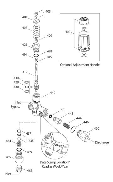
To convert to optional handle assembly, remove items 403 (quantity 2), 410 and 409. Then reassemble as shown in insert.
