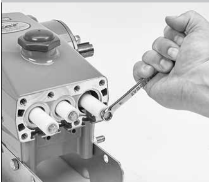
1.22 Using a 10 mm combination wrench, loosen the plunger retainer.
