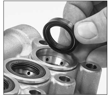
1.45 One side of the low-pressure seal has a groove and spring. Install groove side facing down and press into place.
