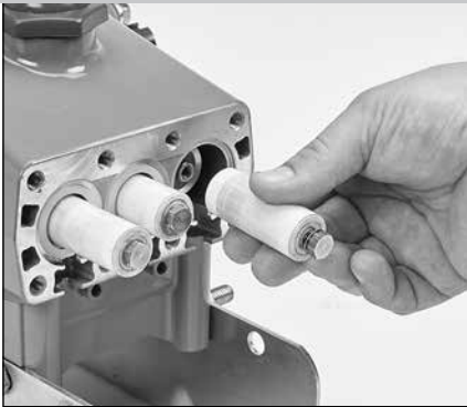
1.19 Remove the plunger and retainer.
