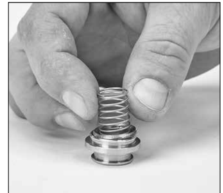
2.15 Place spring onto concave side of valve.
