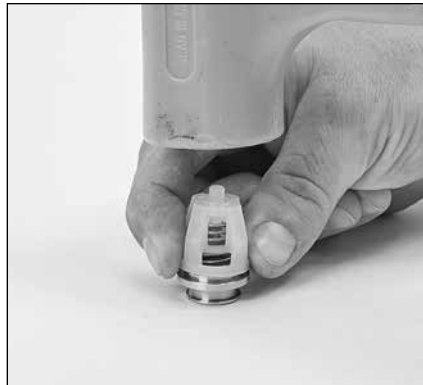
2.17 Using a rubber mallet, lightly tap spring retainer into place.
