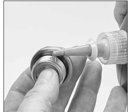
2.22 Place a drop of Loctite® 242® on the threads of valve plug.
