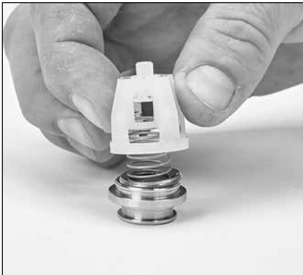
2.16 Place spring retainer onto valve seat.
