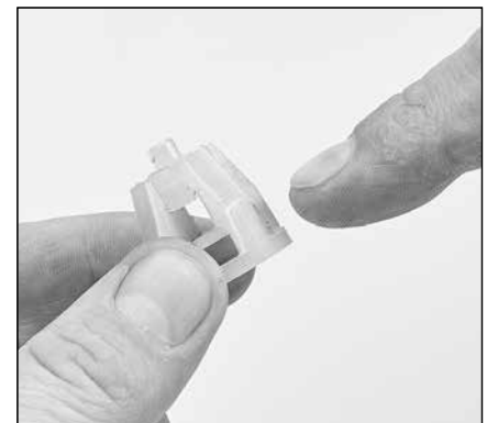
2.07 Inspect spring retainer for cracks, excessive wear or damage.
