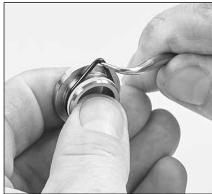
2.11 Using a pick, remove O-ring and backup ring from valve seat.
