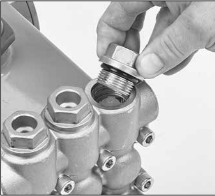
2.23 Install valve plug into manifold and thread by hand.
