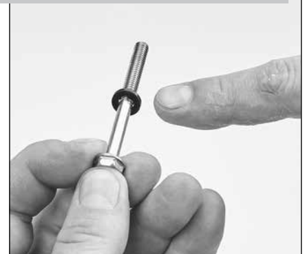
1.24 Remove and inspect seal washer.
