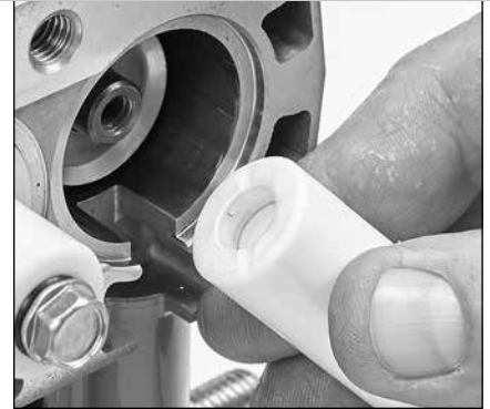
1.35 Look for stepped side of plunger. This side goes towards the pump crankcase.
