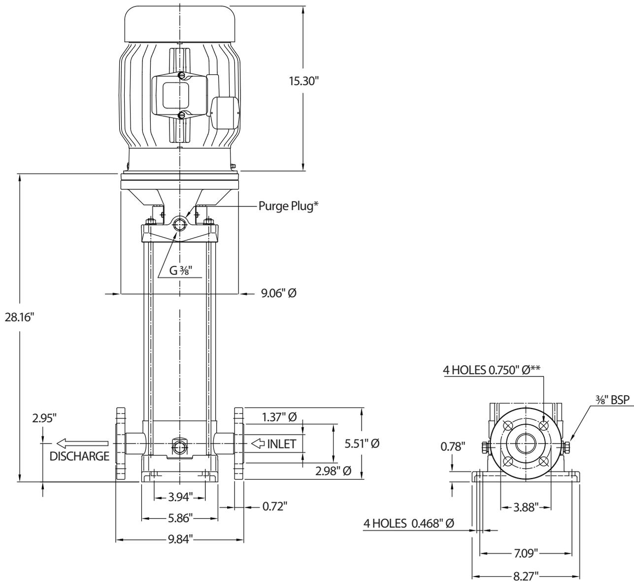
**\* All air must be purged out before operation to prevent seal damage.**
