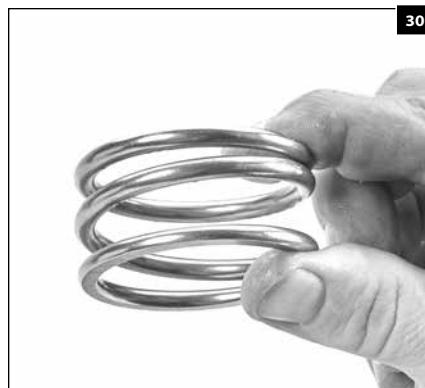
1.24 Inspect the spring for proper tension or any damage.
