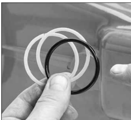
2.05 Inspect for cuts, nicks or damage.
