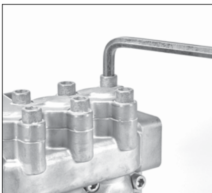
2.37 Using a 12 mm hex wrench, tighten HSH screws using the appropriate cross-pattern for even alignment. Torque to 960 in-lbs, 80 ft-lbs, or 108 Nm.
