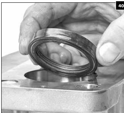
1.104 One side of the low-pressure seal has a groove. Install the groove side facing down and press into place.
