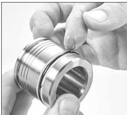
2.32 Apply a lubricant to the outside surfaces of the O-rings and backup rings.
