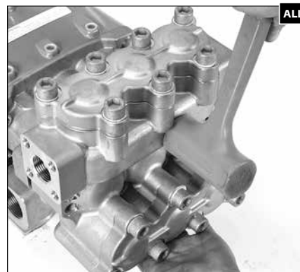
1.160 Lightly tap the manifold with a mallet until resistance from the springs is felt.
