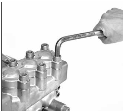
2.01 Use a 12 mm hex wrench to remove the seven (7) HSH screws from the valve plate.
