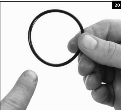
1.16 Inspect for cuts, nicks or damage.
