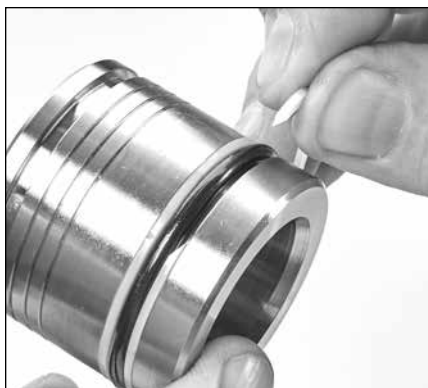
2.31 Install other backup rings below the O-rings.
