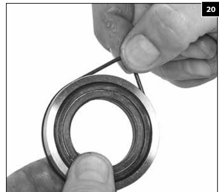
1.96 Replace the O-rings on the low-pressure seal adapters.
