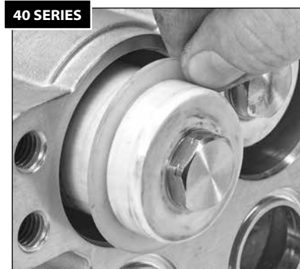
1.142 Install the packing backup rings into the manifold bores.
