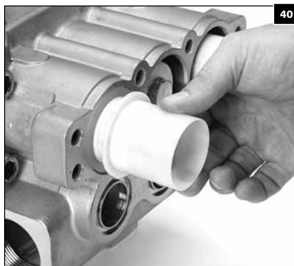
1.143 Install the plunger sleeves over the plungers with the larger diameter end facing the crankcase.
