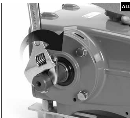
1.35 Rotate the crankshaft with an adjustable wrench to create separation between the manifold and crankcase.
