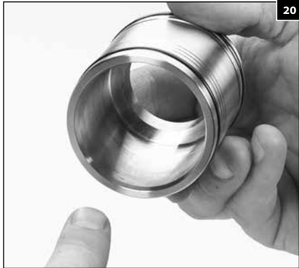
1.12 Inspect the packing cylinder bores to ensure sealing surfaces are smooth and corrosion-free.
