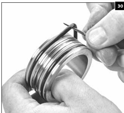
1.19 Using a pick, remove the front packing spacer O-ring and backup rings.
