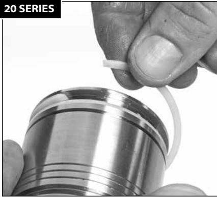
1.113 Install backup rings into the larger groove on the end of the packing cylinder.
