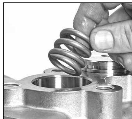
2.06 Remove the coil springs from the manifold.
