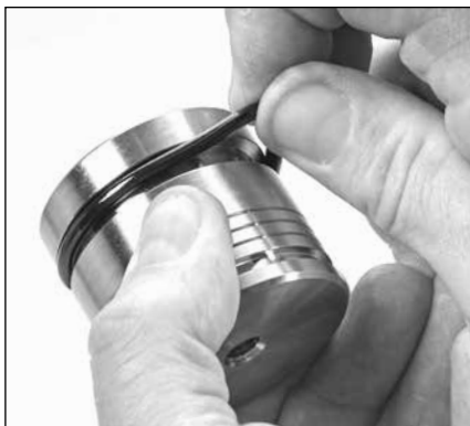
2.29 Replace the valve plug O-rings in the bottom groove of the valve plug.
