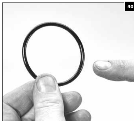
1.28 Inspect for cuts, nicks or damage.
