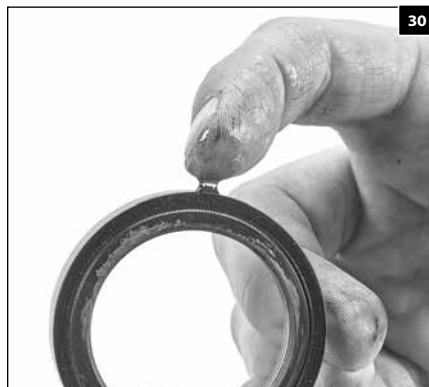
1.100 Apply a lubricant to the outside surface of the low-pressure seals.
