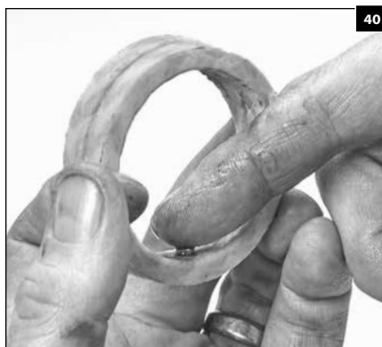
1.146 Apply a lubricant to the inside diameter of the packings.
