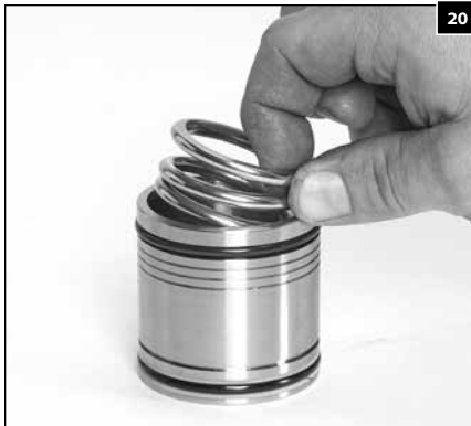
1.116 Install the coil springs into the packing cylinders.
