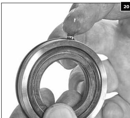
1.97 Apply a lubricant to the outside surfaces of the low-pressure seal adapter O-rings.
