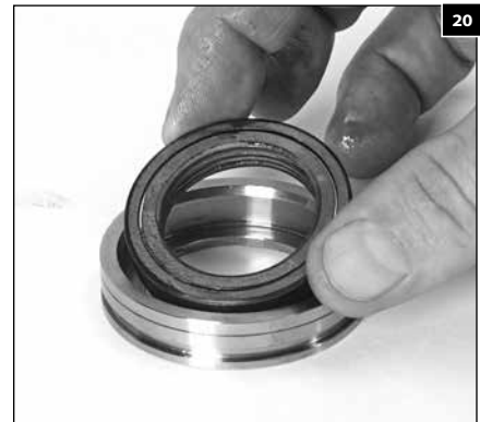
1.93 One side of the low-pressure seal has a groove and a spring. Install the grooved side facing upwards and press it into the low-pressure seal adapter by hand.
