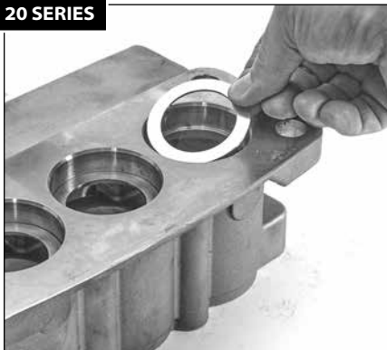
1.91 Install the low-pressure seal washers into the inlet manifold.
