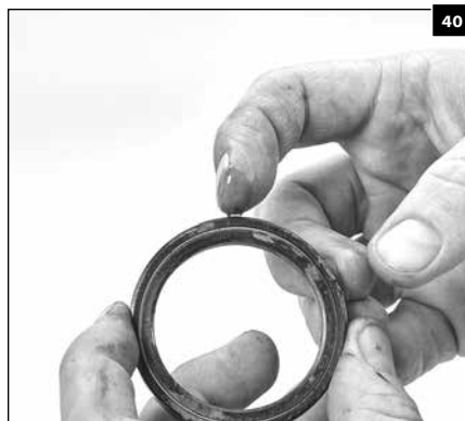
1.103 Apply a lubricant to the outside surface of the low-pressure seals.
