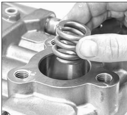
2.28 Install the coil springs on top of the spring washers.
