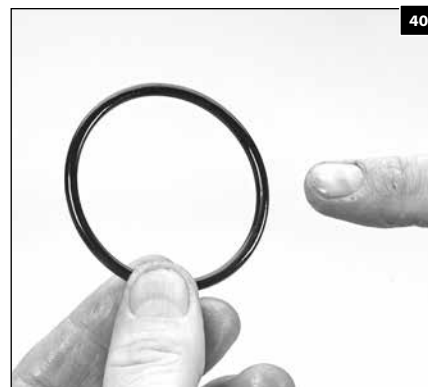
1.30 Inspect for cuts, nicks or damage.
