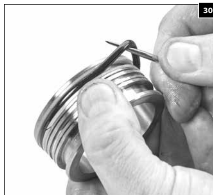
1.21 Using a pick, remove the rear packing spacer O-ring and backup rings.
