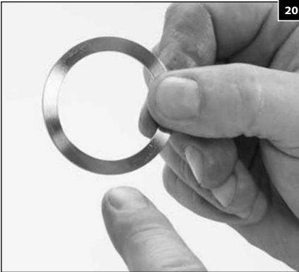
1.11 Inspect the spring washer for wear or damage.
