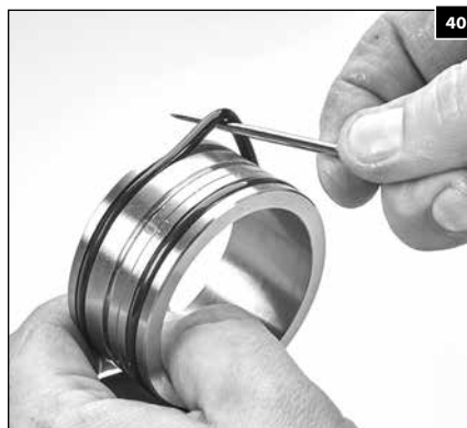
1.27 Using a pick, remove the front packing spacer O-ring.
