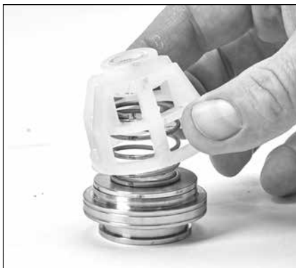
2.22 Place spring retainers onto valve seats.
