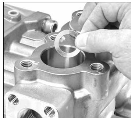
2.27 Install the spring washers on top of the valve assemblies.
