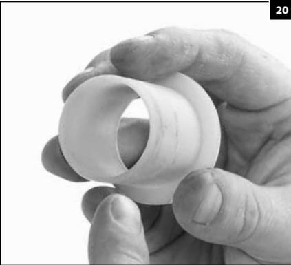
1.10 Inspect the plunger sleeve for wear or damage.
