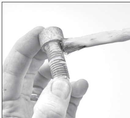
2.35 Apply anti-seize to the threads and underside of the heads of the valve plate HSH screws.
