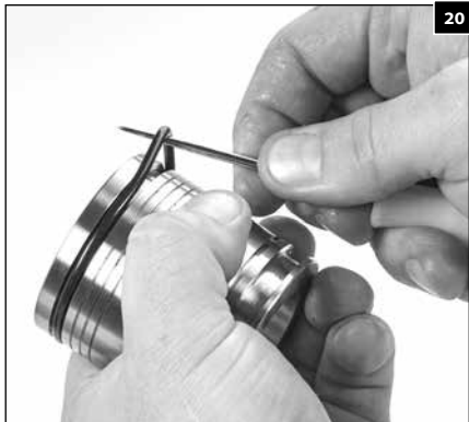
1.15 Using a pick, remove the rear packing cylinder O-ring.
