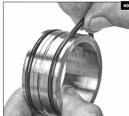
1.154 Install the O-rings into the grooves of the packing spacers.
