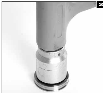
1.95 Using a socket with the same diameter as the low-pressure seals, tap the low-pressure seals all the way into the adapters.
