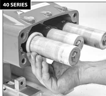
1.102 Install the low-pressure seal spacers onto the seal retainers.
