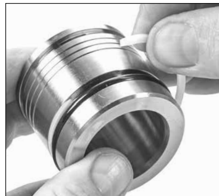
2.30 Install backup rings on top of the O-rings.
