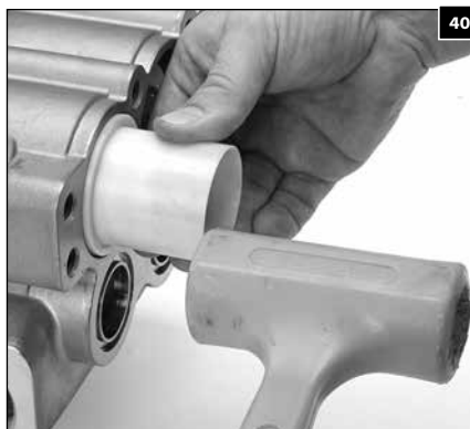
1.144 Lightly tap on the plunger sleeve with a mallet to drive the packing backup ring into the manifold bore.
