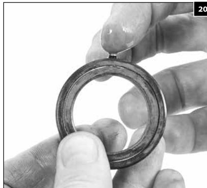
1.92 Apply a lubricant to the outside surface of the low-pressure seals.
