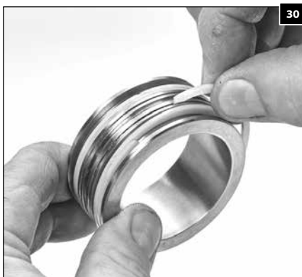
1.138 Install backup rings into the grooves of the packing spacer.
