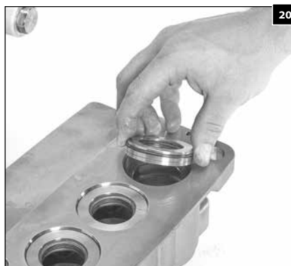
1.98 Press the low-pressure seal adapters into the inlet manifold with the grooved sides of the low-pressure seals facing down.
