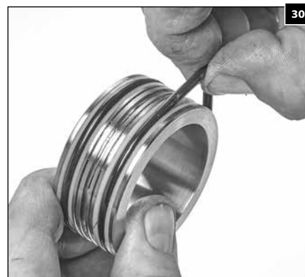
1.139 Install the O-rings between the two backup rings on both ends.
