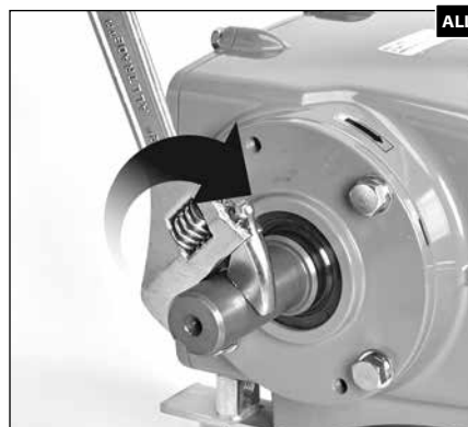
1.165 Rotate crankshaft with adjustable wrench to ensure proper movement of plunger rod assemblies and that seals are not binding.
