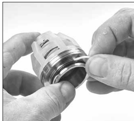
2.24 Replace valve seat O-rings at the top of the groove, then backup rings at the bottom.
