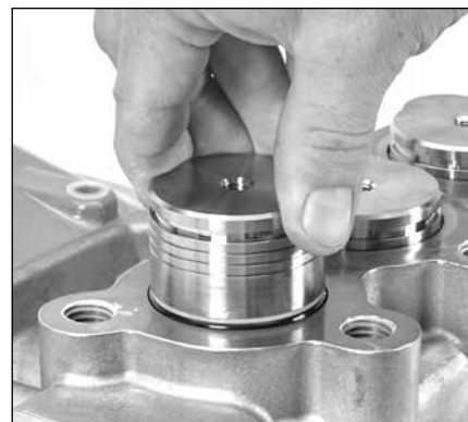
2.33 Press the valve plugs into the manifold bores by hand.
