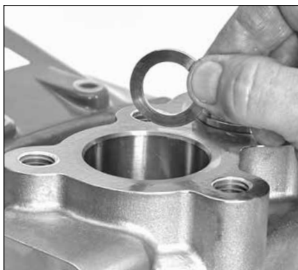
2.07 Remove the spring washers from the manifold.
