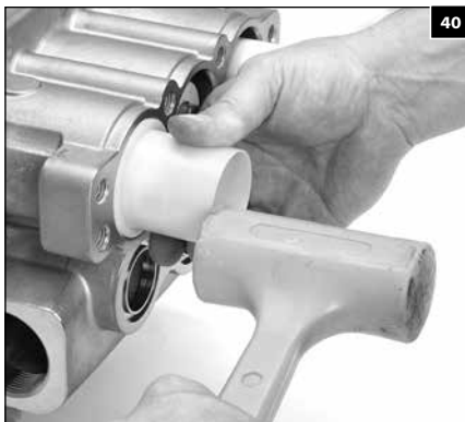
1.150 Lightly tap on the plunger sleeves with a mallet to drive the packings into the manifold bores.
