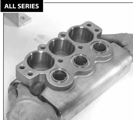
1.105 Flip the inlet manifold over so that the packing cylinder or spacer bores are facing up.
