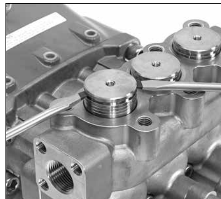
2.03 Insert two (2) flat tip screwdrivers into the grooves on the opposite sides of valve plug and pry upward to remove.
