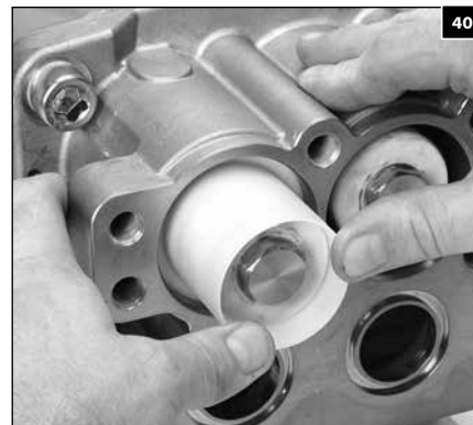
1.151 Press the plunger sleeves into place by hand.
