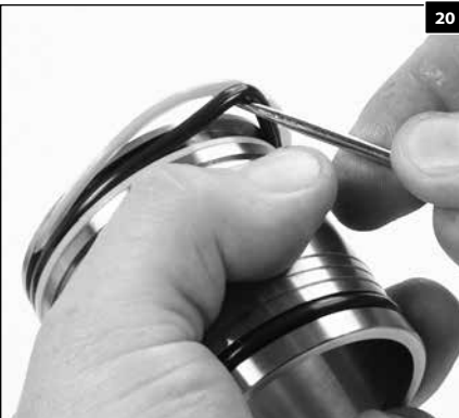
1.13 Using a pick, remove the front packing cylinder O-rings and backup rings.
