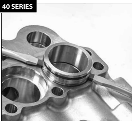
1.25 If the packing spacers remain in the discharge manifold, use two (2) flat tip screwdrivers on opposite sides to pry the cylinders loose from the manifold and remove.
