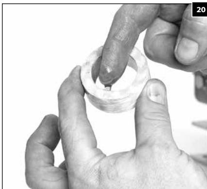
1.119 Apply a lubricant to the inside diameter of the packings.
