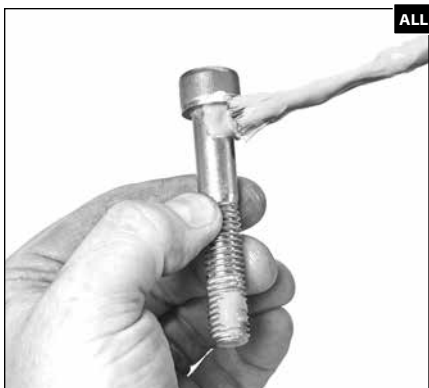
1.161 Apply anti-seize to the threads and underside of the heads of the discharge manifold HSH screws.
