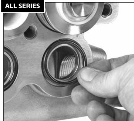
1.157 Install inlet manifold O-rings into the inlet manifold.
