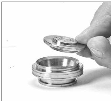
2.20 Place valves onto valve seats with tapered surfaces facing down.
