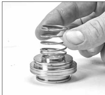
2.21 Place springs onto the concave sides of valves.
