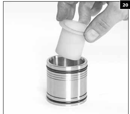
1.118 Install the plunger sleeve into the packing cylinder with the smaller diameter end facing down.
