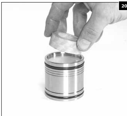
1.120 Install the packings into the packing cylinder.
