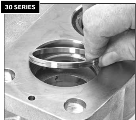
1.99 Install the low-pressure seal spacers into the inlet manifold.
