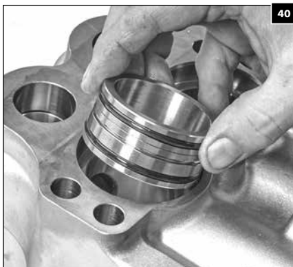
1.156 Press the packing spacer assemblies into the discharge manifold bores.
