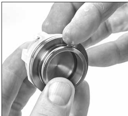
2.25 Apply a lubricant to the outside surface of the valve seat O-rings.
