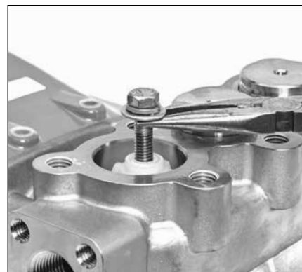
2.09 Use needle-nosed pliers to grasp under the head of the bolt to pull the complete valve assemblies loose from the manifold. Lift up and straight out.
