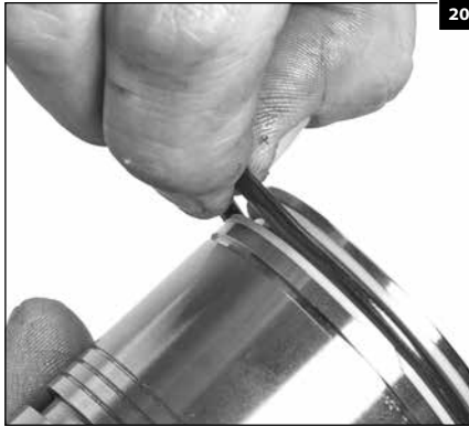
1.114 Install the thicker O-rings between the two backup rings.
