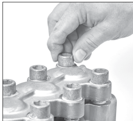
2.36 Install the seven (7) HSH screws by hand.
