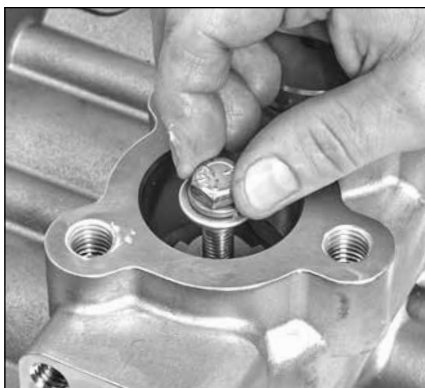
2.08 Thread a 10 mm bolt into the top of the spring retainers.
