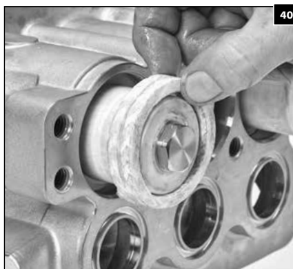
1.147 Install the packings over the plunger.
