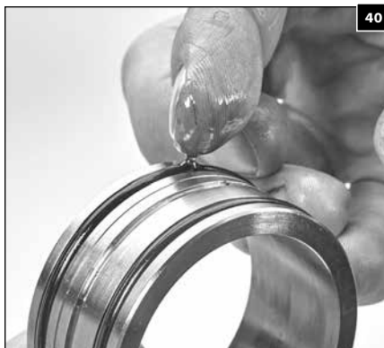
1.155 Lubricate both O-rings on the packing spacers.
