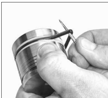
2.04 Using a pick, remove the valve plug O-ring and backup rings.
