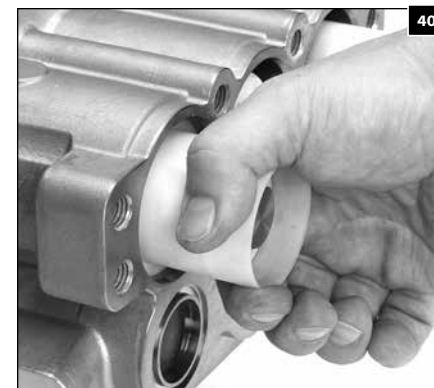
1.145 Remove the plunger sleeve.
