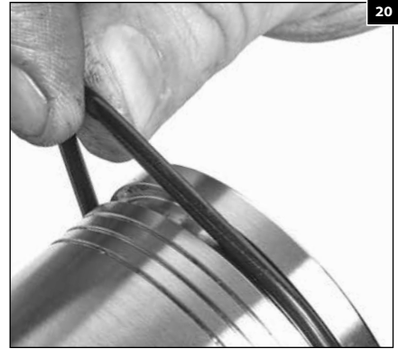
1.115 Install the O-ring into the smaller grooves on the other end of the packing spacers.
