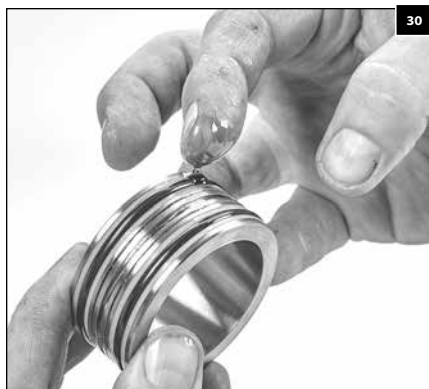
1.140 Lubricate both O-rings and backup rings on the packing spacers.
