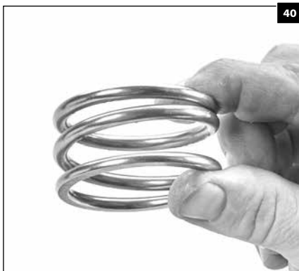
1.32 Inspect the spring for proper tension or any damage.
