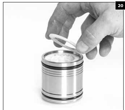
1.121 Install the packing backup ring into the packing cylinder.
