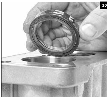
1.101 One side of the low-pressure seal has a groove and a spring. Install the grooved side facing downwards and press it into the inlet manifold by hand.
