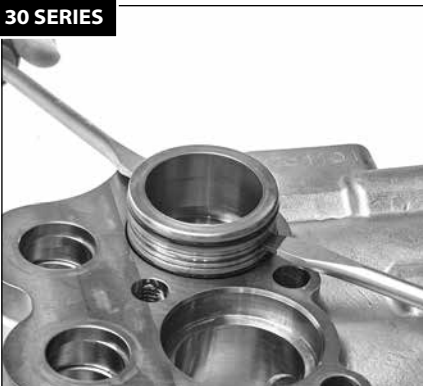
1.17 If the packing spacers remain in the discharge manifold, use two (2) flat tip screwdrivers on opposite sides to pry the cylinders loose from the manifold and remove.
