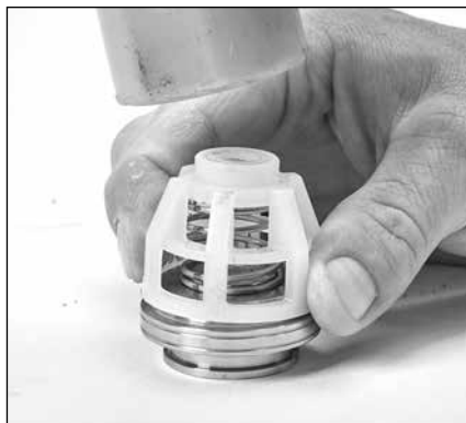
2.23 Using a rubber mallet, lightly tap spring retainers into place.
