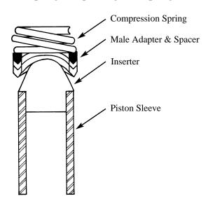
Following are the part numbers for the inserter for the various sleeve-type pumps:
