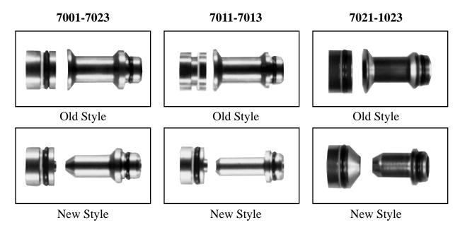
The change was from a flat seating surface to a tapered or cone-shaped surface. The old and new style parts cannot be interchanged.
