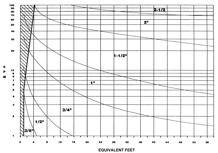
EQUIVALENT FEET = Length of by-pass hose (ft.) + Equivalent feet for fittings in by-pass circuit
