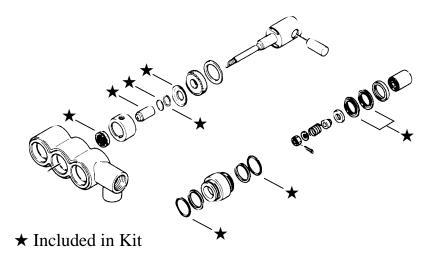
The standard "H" models will gradually be phased out and replaced with this new sleeved "S" version. The standard "H" piston rod will also be phased out. When replacing the "H" non-sleeved piston rod with the "S" sleeved piston rod, it is recommended that all three rods be done as a set. This will assure a uniform performance and provide easier servicing in the future.
