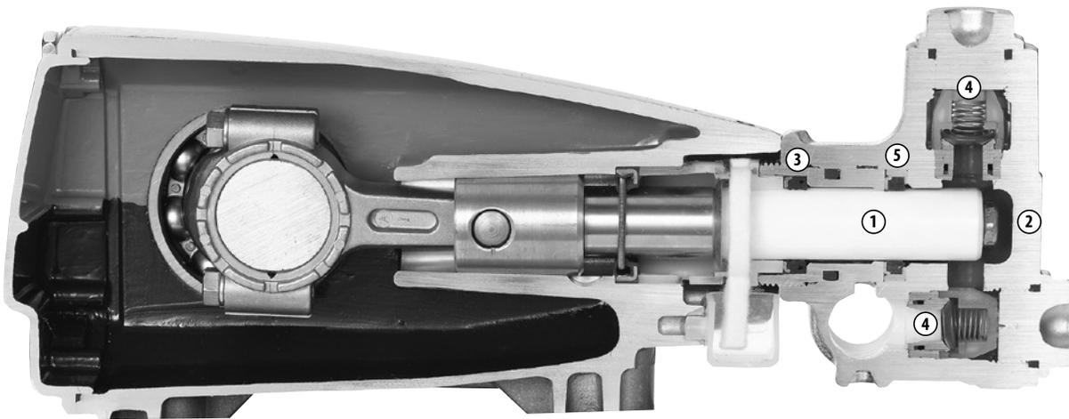
1. Special concentric, high-density, polished, solid ceramic **plungers** provide a true wear surface and extended seal life.
