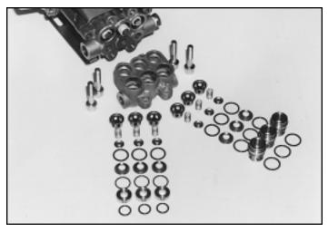
Discharge and Inlet Valve Assemblies
