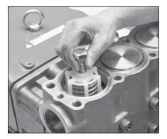
1.5 Use one of the discharge manifold HSH screws (M16 x 120) and hand thread into threaded hole of spring retainer. Grasp M16 screw and pull upward to remove complete valve assembly.
