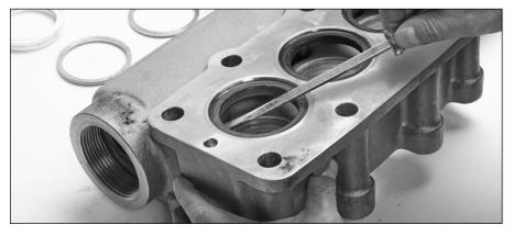
2.20 Turn inlet manifold over so crankcase side is facing upward.2.21 Use a large flat tip screwdriver to remove low-pressure seal from each seal chamber.
