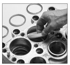
2.17 Remove the pair of white v-packings from each seal chamber.
