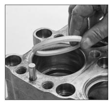
2.25 Install the pair of v-packings in each seal chamber with v-shape facing down.
