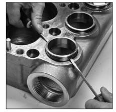
2.7 Carefully insert two (2) flat tip screws into the groove on opposite sides of inlet spacer and pry upward. Do not scratch o-ring sealing area.
