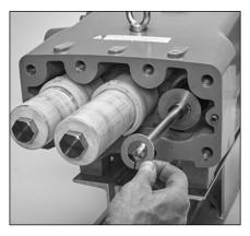
2.45 Slide keyhole washer over plunger rod and position against barrier slinger.2.46 Place a drop of Loctite<sup>®</sup>242<sup>®</sup> on the end of each plunger rod.
