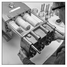
2.15 Remove inlet manifold and place on work surface with crankcase side down.
