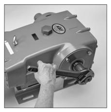
2.13 Use a crescent wrench to turn the pump's crankshaft to assist in separating the inlet manifold from the crankcase.
