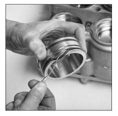
2.5 Use a pick to remove o-rings from both ends of the v-packing spacer.
