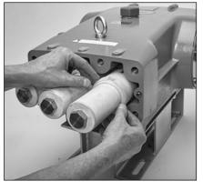
2.49 Slide seal retainer assembly over each plunger rod. Position wick downward.
