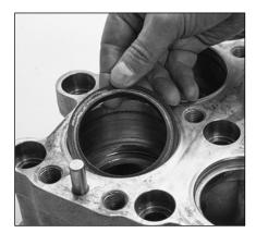
2.24 Install female adapter in each seal chamber with flat surface facing down.
