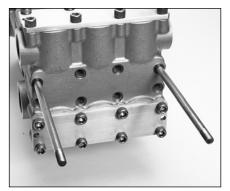
2.1 Hand thread in two (2) M16 x 277 studs (PN 88902). These studs will assist in guiding the discharge manifold over the plungers and evenly distribute the load.
