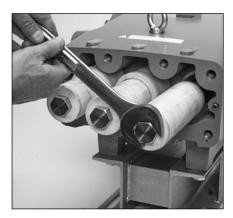
2.33 Use a M30 hex wrench to loosen the plunger retainers.
