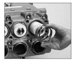
2.9 Remove large coil spring positioned around each plunger.
