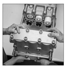
2.3  $\triangle$  Two (2) individuals are required to safely remove the discharge manifold. Place discharge manifold on work surface with spacers facing upward.
