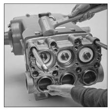
2.14 Use a rubber hammer to tap back side of inlet manifold to further assist in separation from the crankcase.
