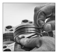
2.29 Install and lubricate o-rings on both ends of inlet spacer.
