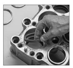
2.18 Remove female adapter from each seal chamber.
