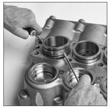
2.4 Insert two (2) flat tip screws into the groove on opposite sides of v-packing spacer and pry upward.
