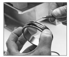
2.8 Use a pick to remove o-ring from the one end of the inlet spacer.
