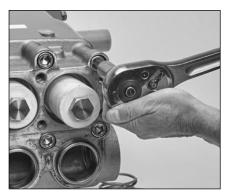
2.10 Use a M14 socket wrench to remove the top outside two (2) M16 x 110 HSH screws on the inlet manifold.
