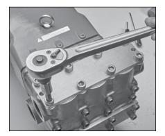
1.0 Use a M14 socket wrench to remove the eight (8) M16 x 30 Hex Socket Head (HSH) screws from the valve plate.
