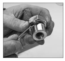
2.38 Use a pick to remove o-ring, backupring and gasket from plunger retainer.
