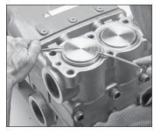
1.2 Insert two (2) flat tip screw drivers into grooves on opposite sides of valve plug and pry upward to remove valve plug with o-ring.
