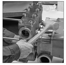
2.2 Use a rubber hammer to tap back side of discharge manifold to separate from inlet manifold.
