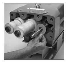
2.36 Remove barrier slinger.2.37 Remove plunger retainer from ceramic plunger.
