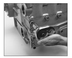
2.0 Use a M14 socket wrench to remove the top outside two (2) M16 x 120 HSH screws on the discharge manifold.
