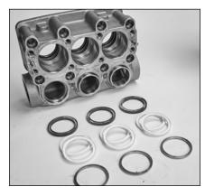
2.19 V-Packing assembly arrangement.
