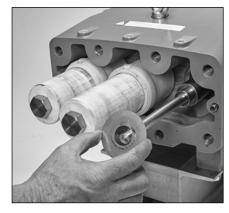
2.44 Slide barrier slinger over plunger rod and position against step on plunger rod.
