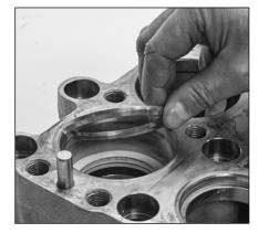
2.26 Install male adapter in each seal chamber with v-shape facing down.
