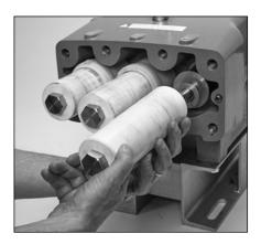
2.34 Grasp ceramic plunger and turn counterclockwise to remove plunger from plunger rod.
