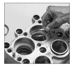
2.16 Remove male adapter from each seal chamber.
